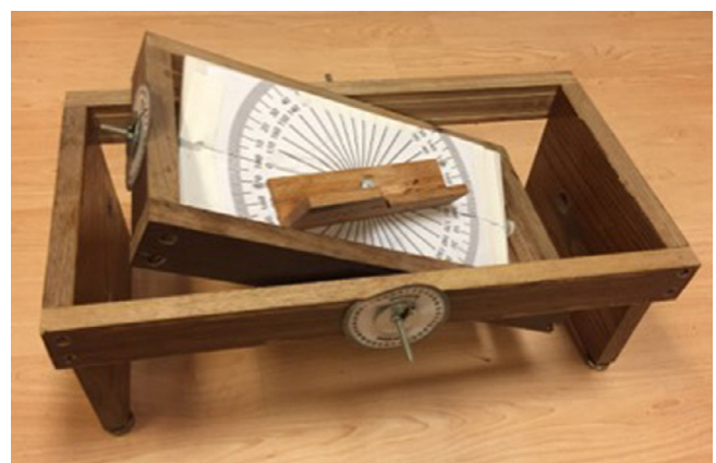
FIGURE 1 Triplanar jig used to position cadaver femurs during radiograph acquisition. The jig allows controlled rotation/angulation in frontal, axial, and sagittal planes. Protractors fixed at the axes of rotation allow for precise quantitation of axial rotation and frontal and sagittal plane angulation
