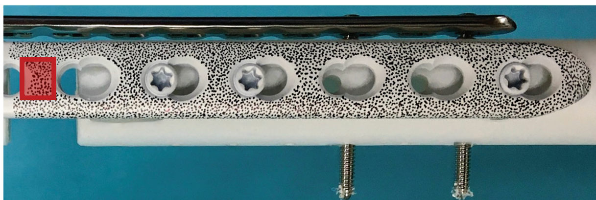
Fig. 3 Primary plate speckle pattern used for three-dimensional digital image correlation strain measurement. Strain measurement was performed at the axial plate region between the central screw holes, overlying the fracture gap (rectangle).
