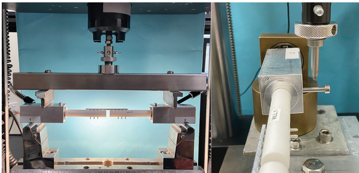
Fig. 2 Biomechanical testing setup for four-point compression bending (left) and torsion (right).
